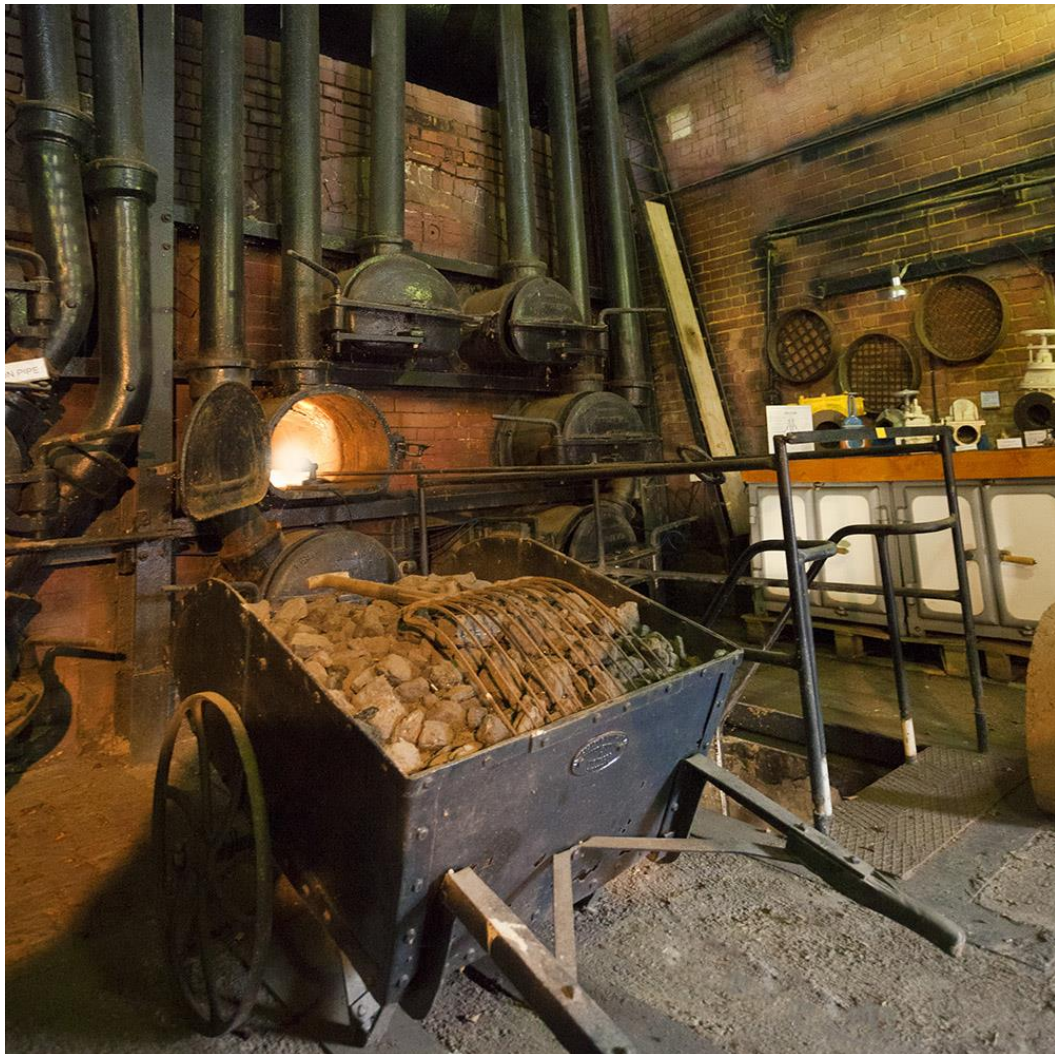
Illustrative picture of the inside of a retort house with horizontal gas retorts. Fakenham gas works. Source: Fakenham Gasworks Museum. Available at https://fakenhamgasmuseum.com/
